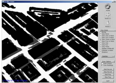
Fig. 2. The satview tool. All areas that can see three or more satellites are shown in white
