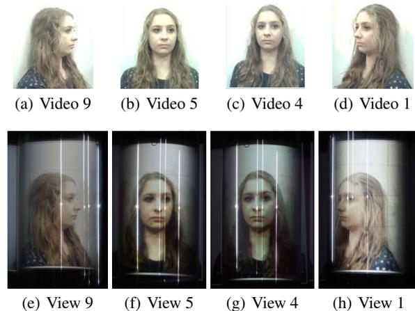
**Figure 1.** The remote person is gazing at target 5. The top row is four videos simultaneously captured from four different cameras. The bottom row is four photos of the same display from four different perspectives. See Figure 2 for camera, target and viewpoint numbers.
