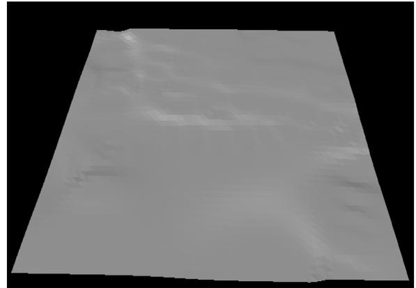
**Figure 4 Smooth surface created by interpolating the LIDAR data by the inverse distance weighting function**
