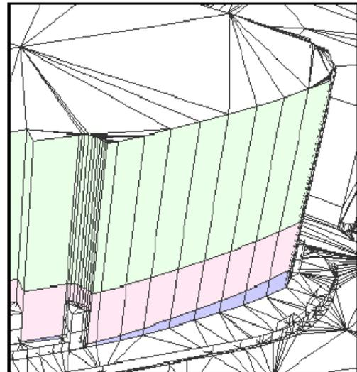
**Figure 5 Triangles comprising a building façade**
