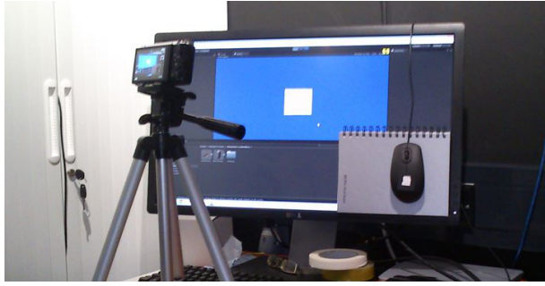
Fig. 1. Example setup for the Automated Frame Counting method. The mouse is the tracker and the VE is a Unity set.
