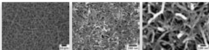
Above: Scanning electron micrographs of materials currently being considered for laser generated ultrasound, including electrospun fibres with integrated carbon nanotubes (left), and functionalised multi-walled carbon nanotubes dip-coated on a glass substrate (centre and right).
