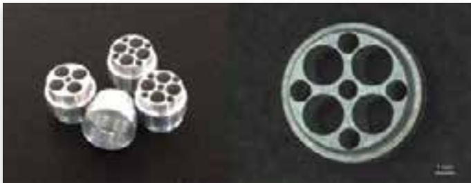
Above: View upon components of the dual-segment fluidic-actuated instrument produced at KUL through precision manufacturing techniques.
