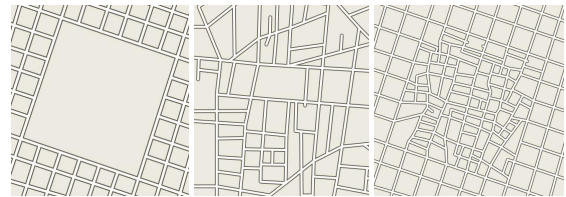
Figure 3: We fill in a hole in a grid pattern (left) with real world irregular streets, and get a new, well connected street network (right). The synthesis starts from the nodes on the boundary of the hole, which are manually marked as unfinished .
