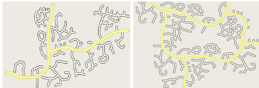
Figure 6: Left: Input a real road network (South Woodham Ferrers, UK) with major and minor curved roads. Right: Starting from a random initial node, our method arrive a road network that resembles the input.
